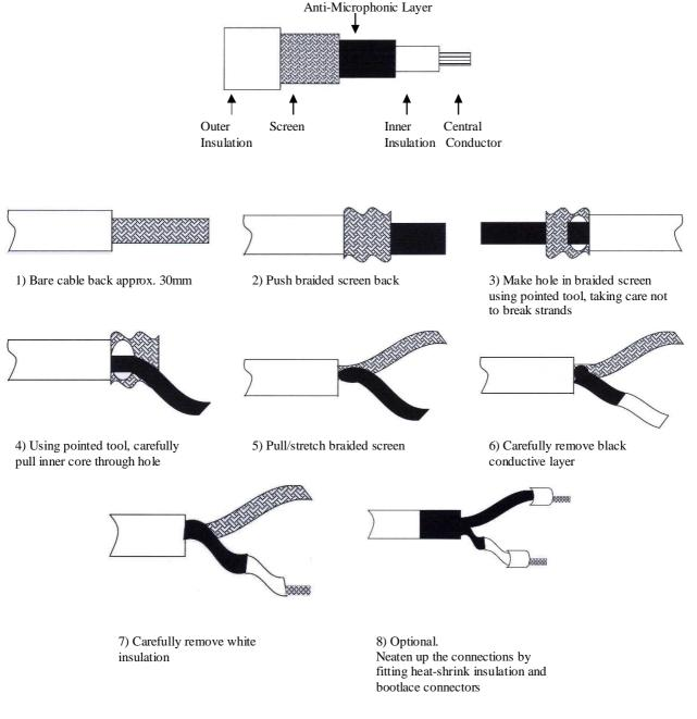
Most electrode are supplied with a BNC connector fitted. It is often necessary to remove the BNC connector or shorten the cable suitable for connecting to screw terminals.
